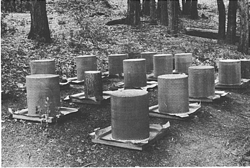
Figure 4. Method of forcing attacks of ips on sprayed bolts treated with lindane and dieldrin surface and tissue deposits
